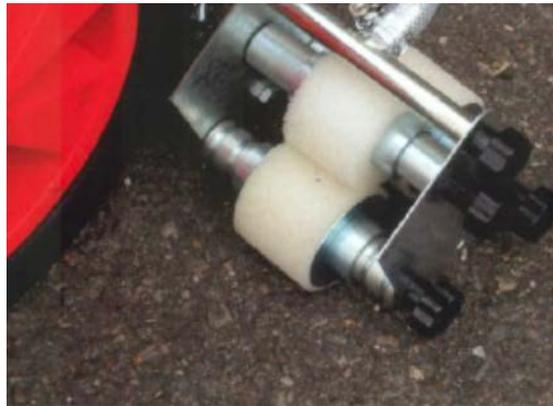
Place all components apart from plastic retaining nut and feed hose in a full bucket of cleaning fluid and clean using a stiff brush. Tank should be flushed out with cleaning fluid and a drop of oil inserted in the control tap to prevent seizure. Do not place feed hose in cleaning fluid. Allow paint to dry inside hose and flex hose, and when dry, to remove.
