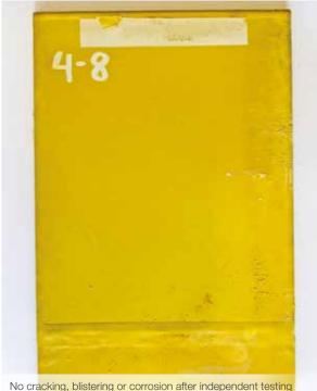
No cracking, blistering or corrosion after independent testing in seawater at over 160°C (320°F) after extended duration
