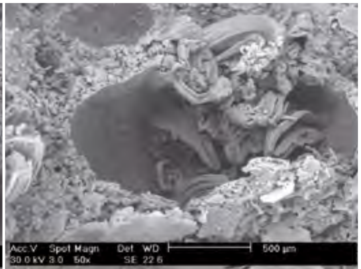
PHOTO 2 - Crystallisation of salts in the macropores of dehumidifying mortar from the MAPE-ANTIQUÉ range
