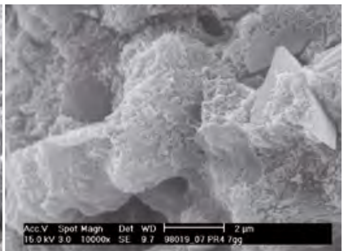
PHOTO 4 - Micrograph of MAPE-ANTIQUÉ mortar after 8 days of "ageing". Notice the rounded structure typical of a stabilised system
