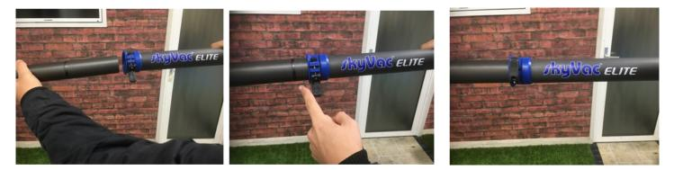
Open clamp and insert pole, up to the positive stop marking and no further. Adjust tension of the clamp and close.
