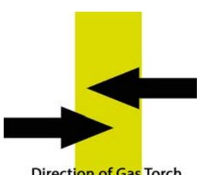
Hold the gas torch 4 to 6 inches above the Kestrel Overbanding Tape. Starting at one end while constantly moving the flame in a short side to short side motion (as shown opposite) to gradually heat up the material. Always work from side to side as shown rather down the length of the material.
