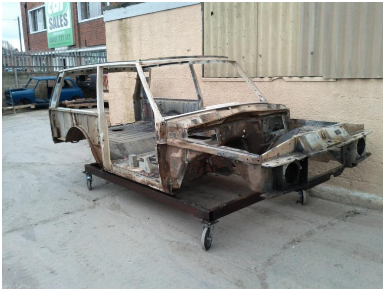
Paintwork is removed by burning
