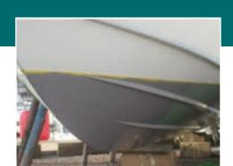
After this you can apply Teamac Marine Undercoat and Gloss as appropriate. For a higher performance system use either Metaclor Primer followed by Chlorvar Topcoat or Epidox 2 pack Zinc Phosphate Primer followed by P101 Topcoat.
