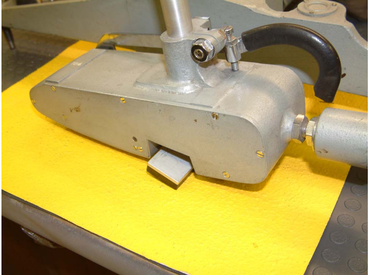
Plate 1 Sample 1 being tested for slip resistance
