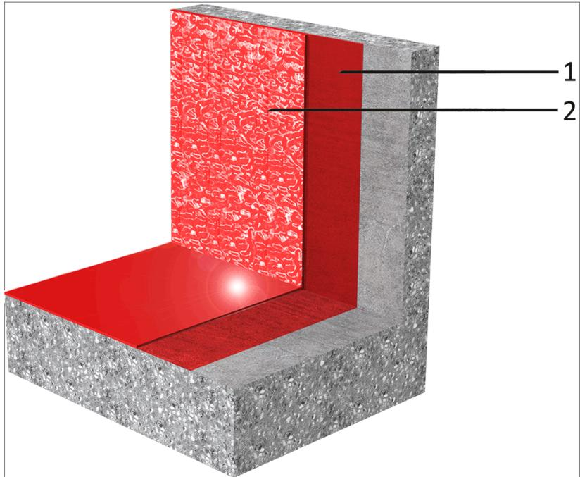
**Sikafloor® MultiDur ET-31 V system (~ 1.5–2.0 mm)**
