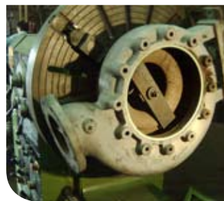
Pump case repaired and rebuilt using Scotchkote Epoxy Ceramic Rebuild EG 513. A second coat of Scotchkote Epoxy Ceramic Surfacers FG 512 applied for a smooth friction free finish.
