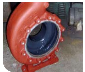
Pump case repaired and rebuilt using Scotchkote Epoxy Ceramic Rebuild EG 513. A second coat of Scotchkote Epoxy Ceramic Surfacers FG 512 applied for a smooth friction free finish.
