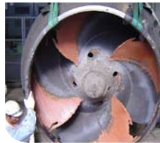
Pump impeller refurbished by rebuilding with 3M™ Scotchkote™ Epoxy Ceramic Rebuild EG 513 to repair corrosion damage followed by 3M™ Scotchkote™ Epoxy Ceramic Surfacers FG 512 for a smooth finish.
