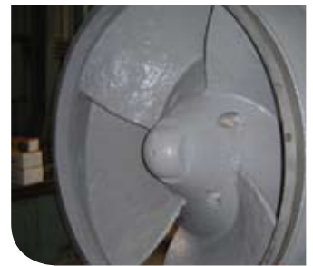
Pump impeller refurbished by rebuilding with 3M™ Scotchkote™ Epoxy Ceramic Rebuild EG 513 to repair corrosion damage followed by 3M™ Scotchkote™ Epoxy Ceramic Surfacers FG 512 for a smooth finish.
