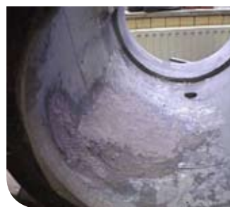
Corroded and eroded pipe shown after blast preparation and then shown fully protected with an application of Scotchkote Epoxy Ceramic Surfacers FG 512.
