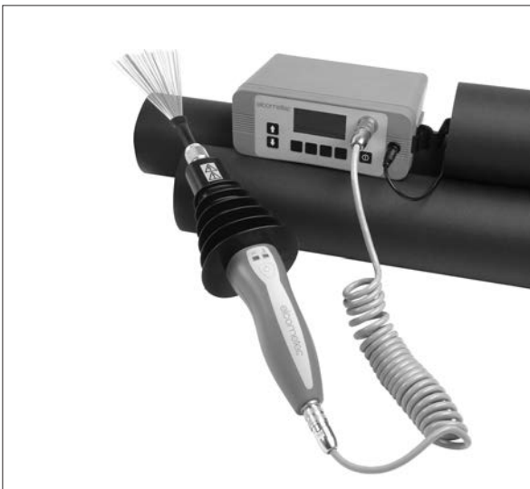
Image 8.2 Porosity probe for the tests under ISO 2746.
